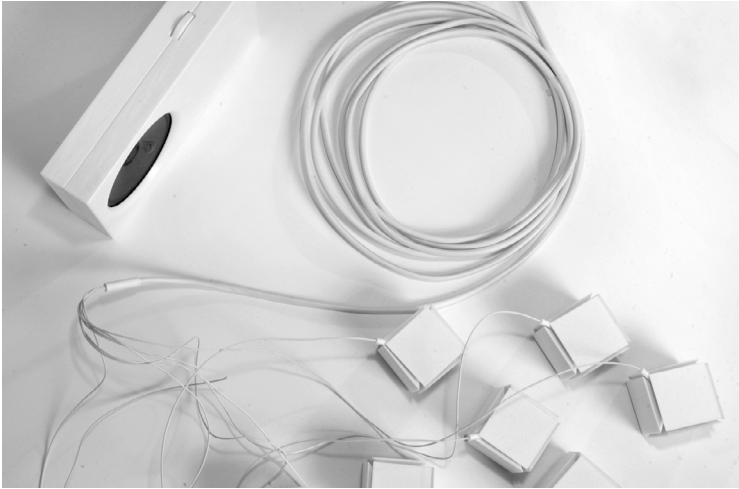
FIGURE 2.2 Radio, cables, and piezo-electric terminals. (Photo by Diego Combina)
